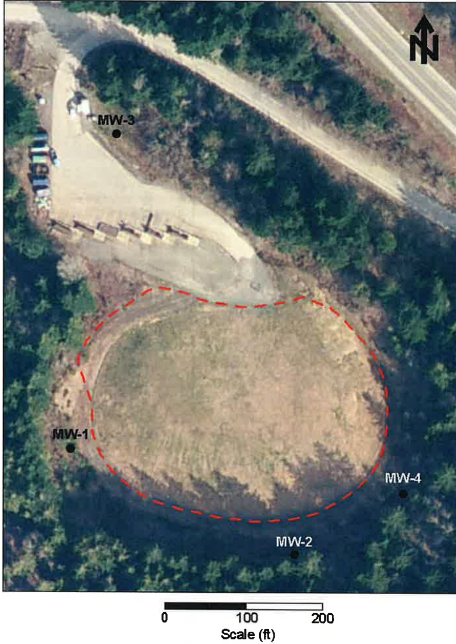
Figure 2. Monitoring Well Location Map.
